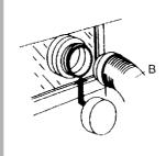
With a stacked dryer the hole in the window should ideally be made below the vent.
